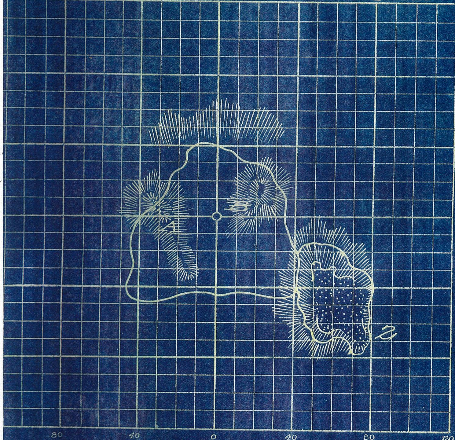
While it is desirable to have a clear view of Green, it is not essential, so if the cut or fill entails too much work leave the putting surface blind.
