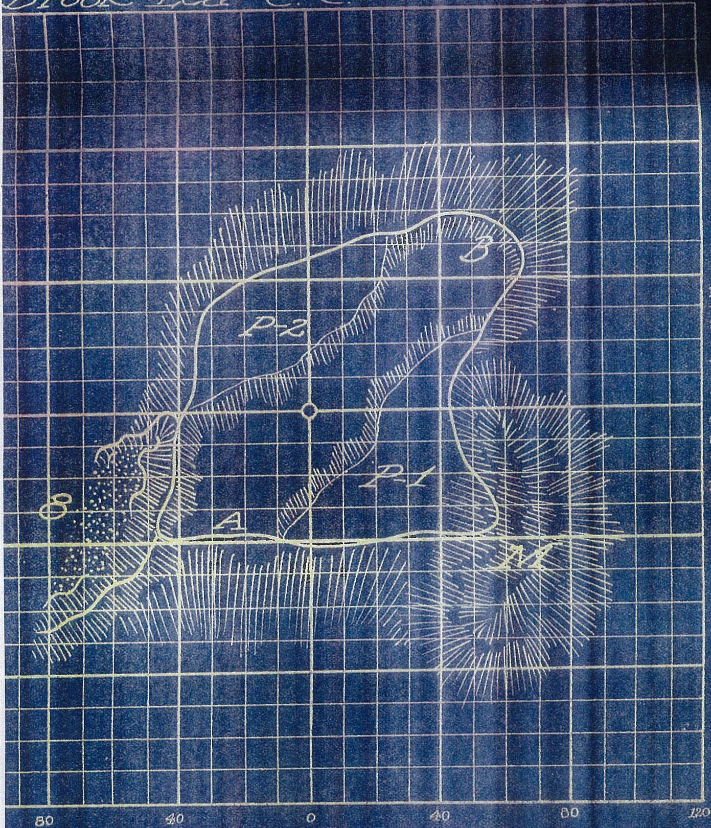
Body of green raised not less than 1 ft. in front at A and 2 ft. 6 in. at B.
