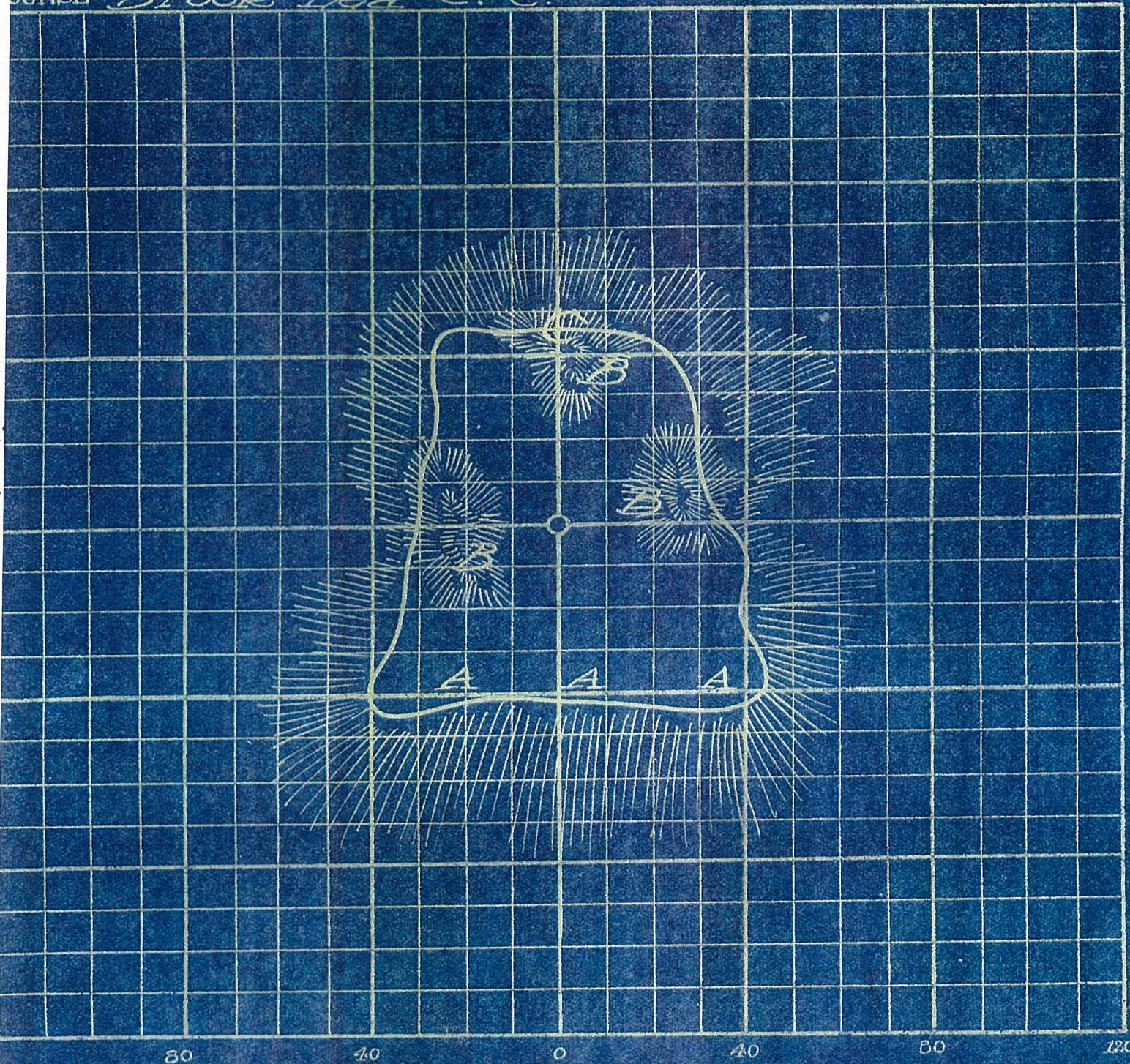
Front edge at A lowered and rear at C raised sufficient to have all the surface of green clear in view from the 225 yd. mark.
