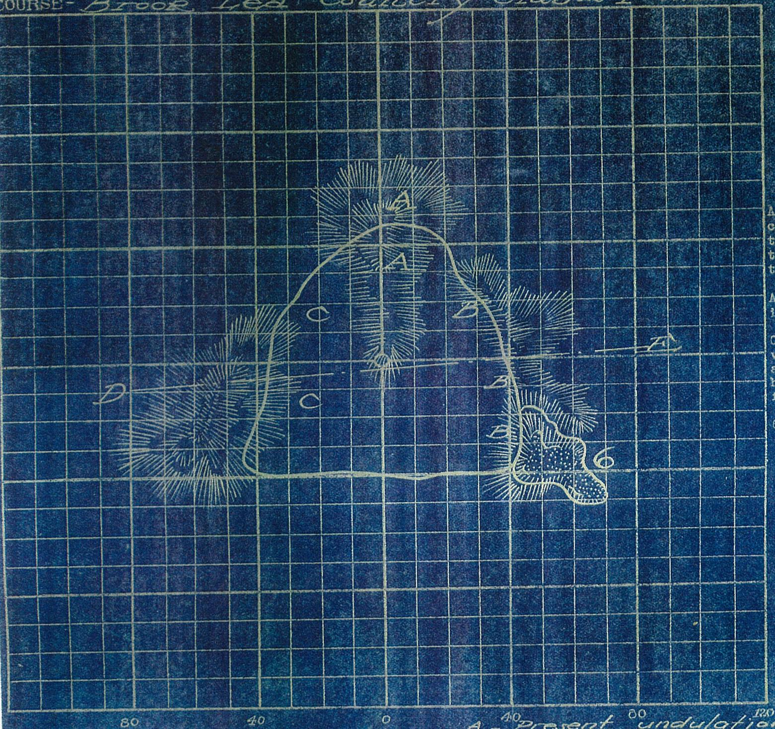
A is present undulation, no change unless found necessary that it should be raised so as to be clearly in view from the tee and from the 200 yd. mark.
